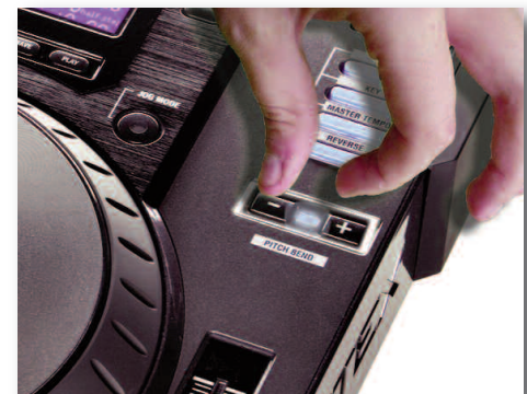
Fig 8.3 - Pitch On/Off by pressing both buttons simultaneously. If in Master Tempo Mode doing this will return the unit to Pitch.
