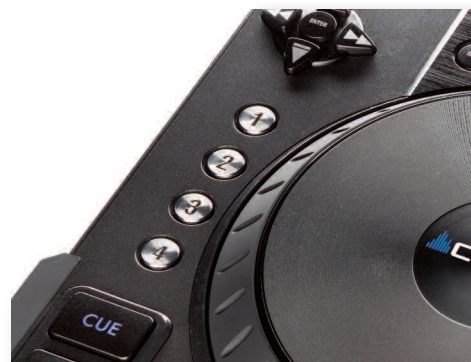
Fig 13.2 - Choose a number for your loop and press the button twice, once to enter the start point and once to enter the end point. To exit press Shift+the loop number, and to reloop press the number again.
