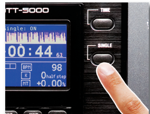
Fig 5.3- Use the Single button to toggle between Single on and Single off mode
