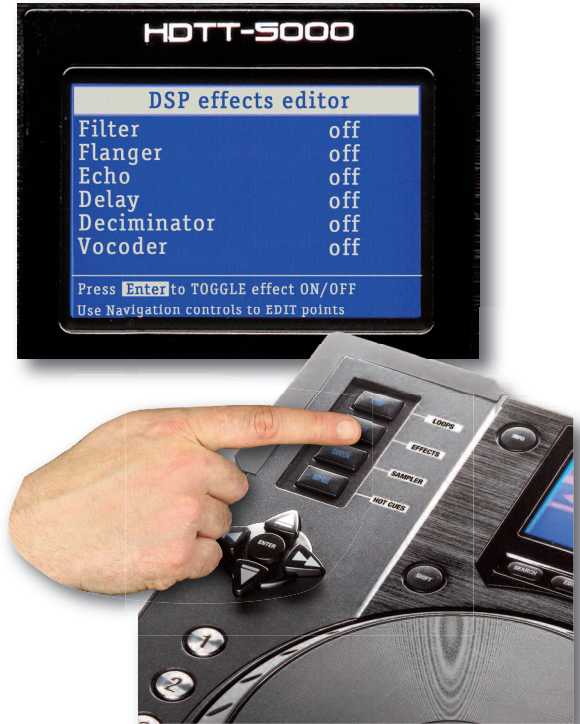
Fig 14.1 - Entering the DSP Menu. Press the DSP button twice to use DSP effects from the Play screen.
