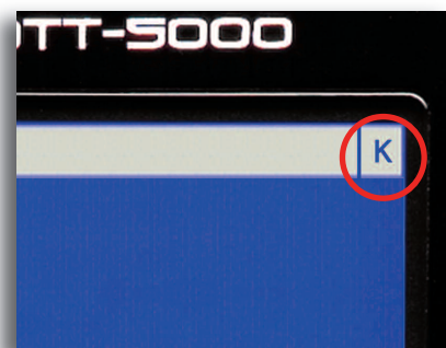
Fig 4.0 A small letter (K) identifies which HDTT-5000 is being controlled with the USB Keyboard
