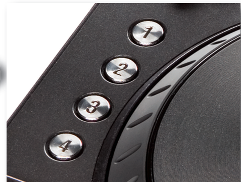
Fig 15.2 - Choose a number and press the chosen button to record the start point of a sample.. Press it again to record the out point, at which point the sample will engage. To exit, press shift plus the number of the sample. To delete, press shift plus the number again.
