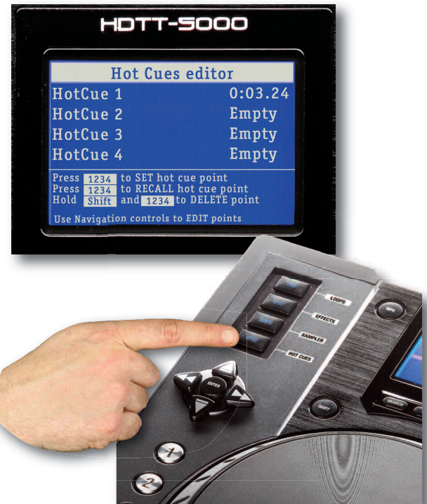
Fig 12.1 - Entering the Hot Cue Menu. Press the Hot Cue button twice to use Hot Cues from the Play Screen. Using Hot Cues from the Play Screen is the same as in the Cue Menu.
