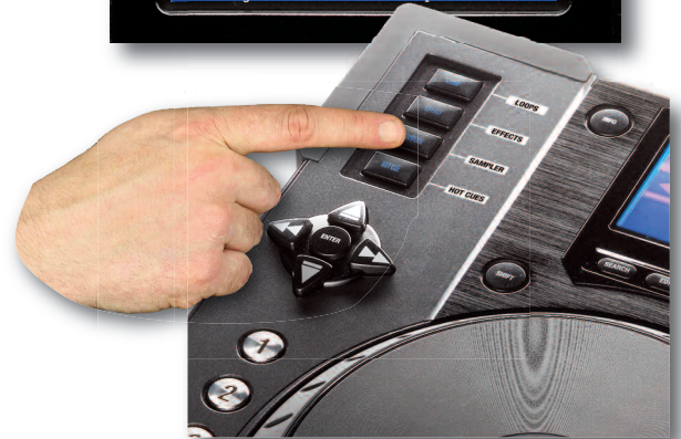
Fig 15.1 - Entering the Sample Menu. Press the Sample button twice to use Loops from the Play screen. Using Samples from the play screen is the same as from the Sample menu.
